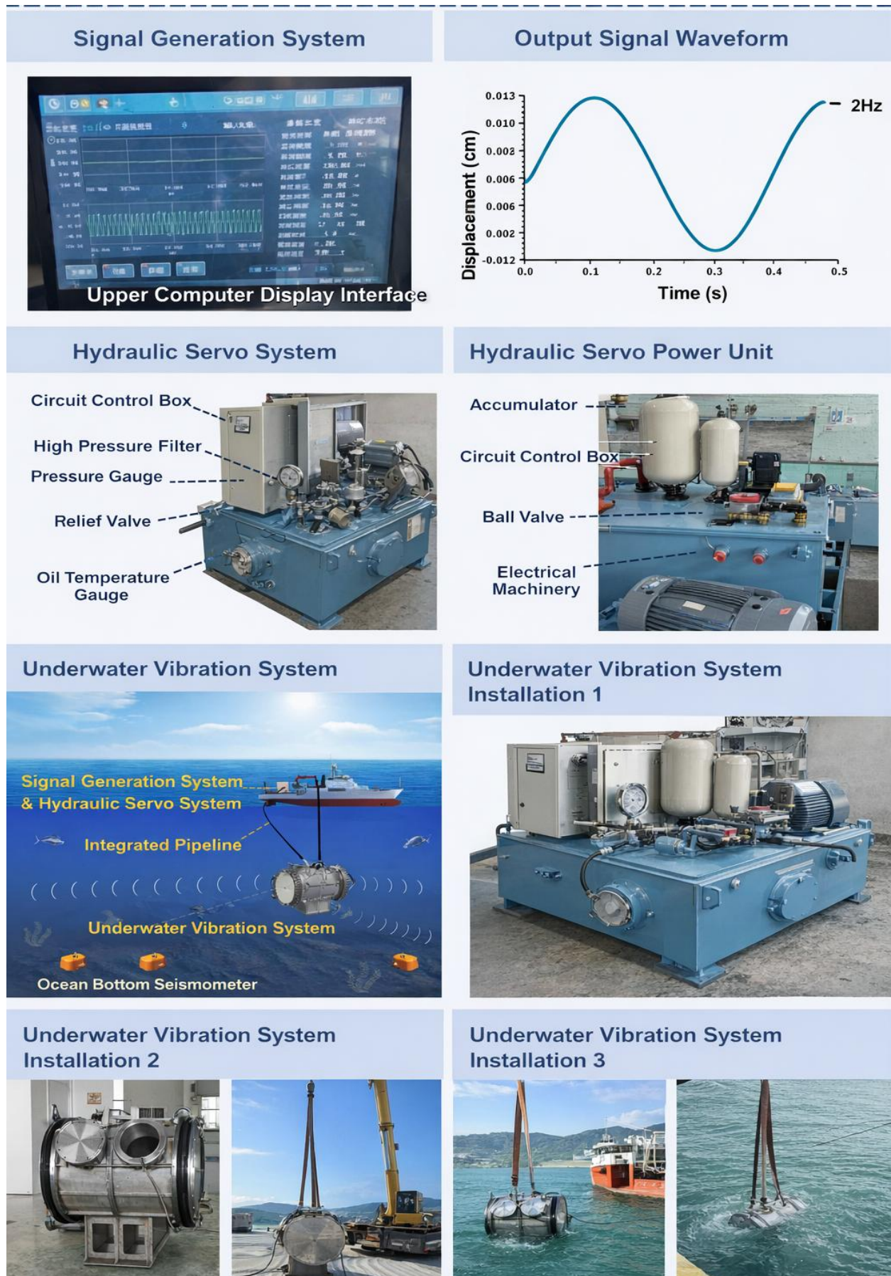
Figure 1 – Configuration of an underwater vibration excitation and measurement system
